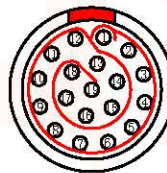
Welded surface (焊接面)
