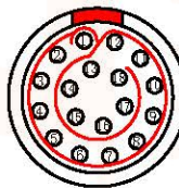
Welded surface (焊接面)
