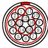
Welded surface (焊接面)
