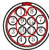
Welded surface (焊接面)
