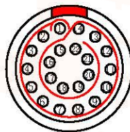
Welded surface (焊接面)
