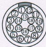
Welded surface (焊接面)
