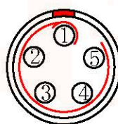
Welded surface (焊接面)
