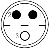
Welded surface (焊接面)
