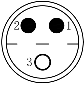
Welded surface (焊接面)
