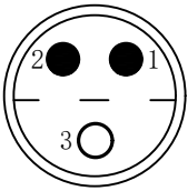
Welded surface (焊接面)
